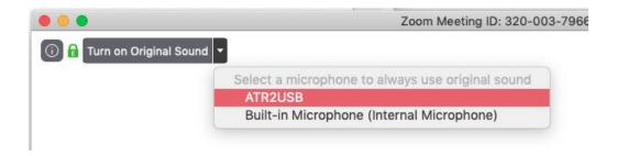
4. SELECTING STETHOSCOPE - To send the Thinklabs One stethoscope sound to the remote listener, <u>Click</u> the ^ arrow to the right of the mute microphone icon. Then select the ATR2USB in the popup menu in the "Select a Microphone" Section
